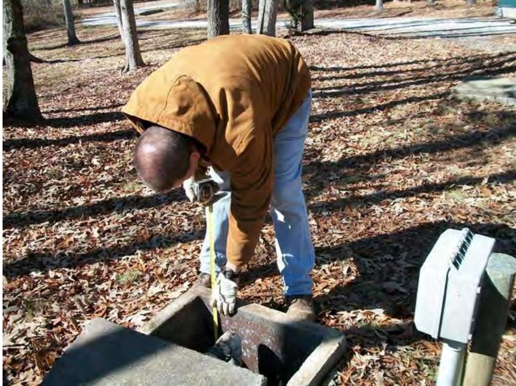
Measuring Pump Flow Rate
