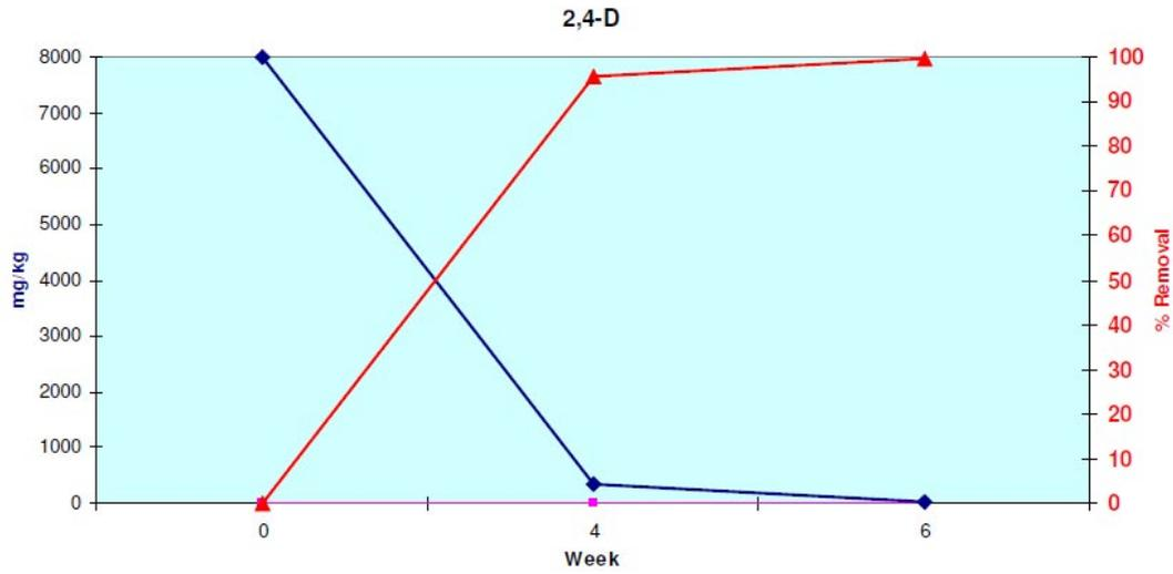
*\* It was observed that high levels of contamination remained in large clay bodies indicating that these need to be crushed prior to treatment.*
