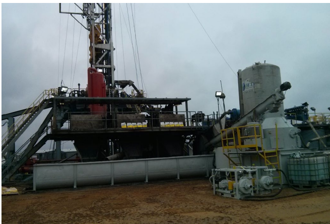
Rig setup: raw cuttings from shakers, dryer and BiOWiSH® treatment totes
